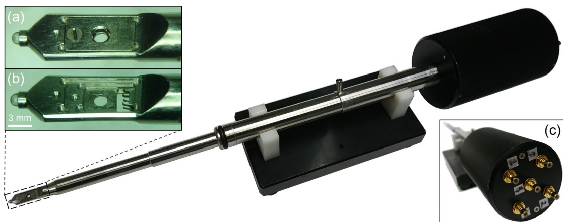
Figure 1.6: Microchip TEM Holder. (a) Holder tip with cover affixed and (b) removed with electrical pins visible. (c) Backside of holder with electrical interconnect plugs.
