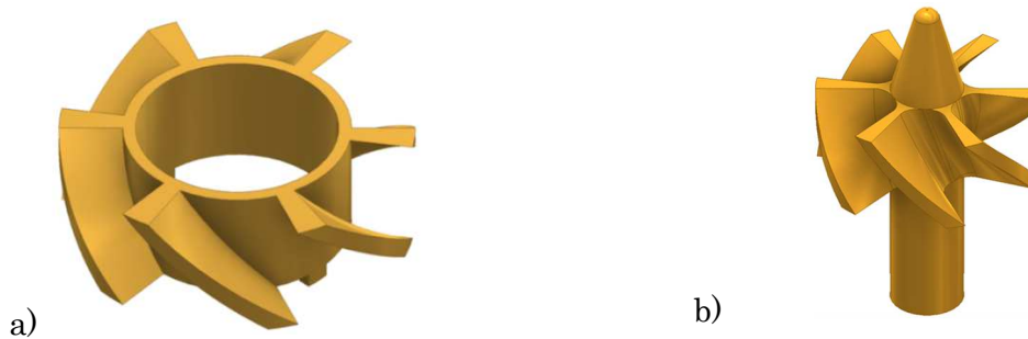
Figure 6: swirler for an airblast injector configuration a) example for an outer swirler; b) example of an inner swirler
