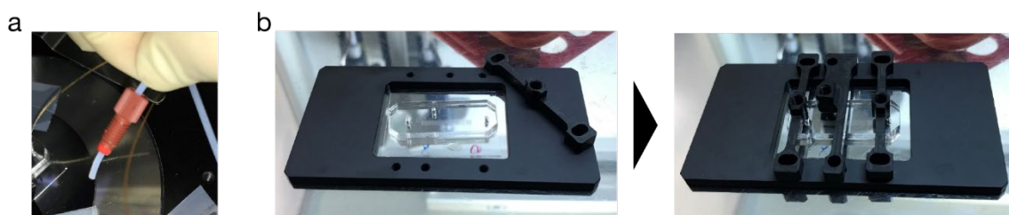
Figure 2. 8 Pictures of the setup of tubes and the arraying device. (a) A typical setting of tubes connected to the arraying device. The fused silica capillary was sleeved by an ETFE tube. (b) Housing structure for the stabilize and reproducible connection.
