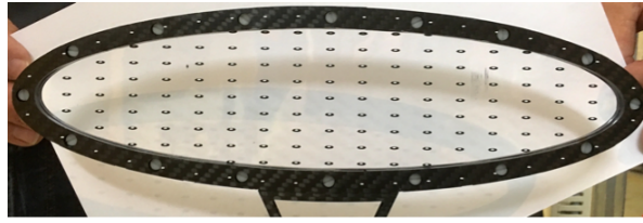
Figure 1.9 Muon stopping target for MEG II (width:270 mm, height:66 mm) [7].
