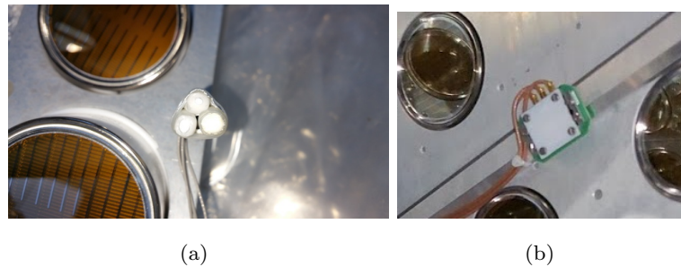
Figure 2.26 LEDs for photosensor calibration [34]. (a) LEDs on the lateral face. (b) LEDs on the outer face.
