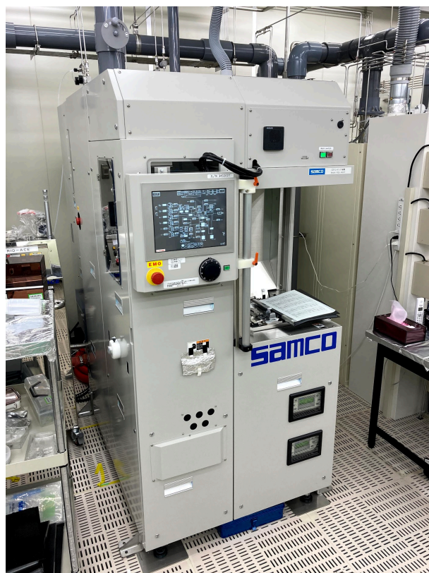
Figure 4.7: Photography of the ICP RIE machine used in this study (RIE-140iP).
