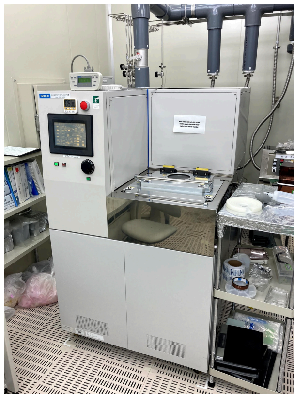
Figure 5.5: Photography of the ICP RIE machine used in this study (RIE-200iP).
