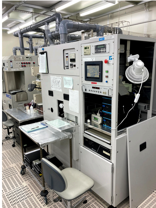
Figure 8.5: Photography of the ICP RIE machine used in this study (RIE-101iP).
