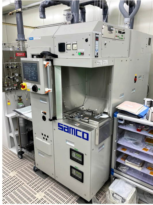
Figure 6.3: Photography of the ICP RIE machine used in this study (RIE-140AI).
