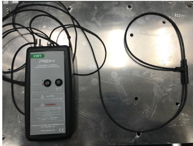
Figure 3.41: Current transformer. The current flowing inside the loop at the right side of the picture is converted to voltage signal.
