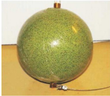
Figure 3.24: Picture of the NiCf source, which is made of 6.5 kg of NiO and 3.5 kg of polyethylene. The Cf source is located inside the ball and provides neutrons. Taken from [42].
