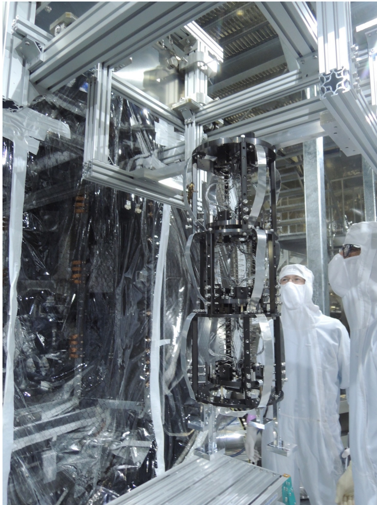
Figure 7.2: HLVIS was mounted on a cart on the installation frame for movement into the cryostat at IXC.
