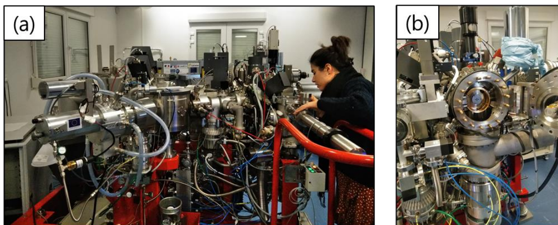
Figure 2.14. (a) High-resolution SIMS (1280 HR2) installed at Centre de Recherches Pétrographiques et Géochemiques, and (b) a sample chamber of the SIMS.
