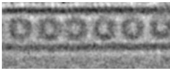
Figure 2.2. A TEM image of C 60 @CNT (62.5 ms/ frame, 80 kV, EDR = 22 \times 10^5 e - nm -2 s -1 ). Scale bar: 1 nm.
