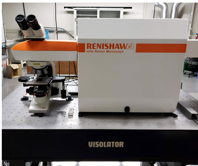
Figure 2.6 Photograph of the equipment used in microscopic Raman spectroscopy.
