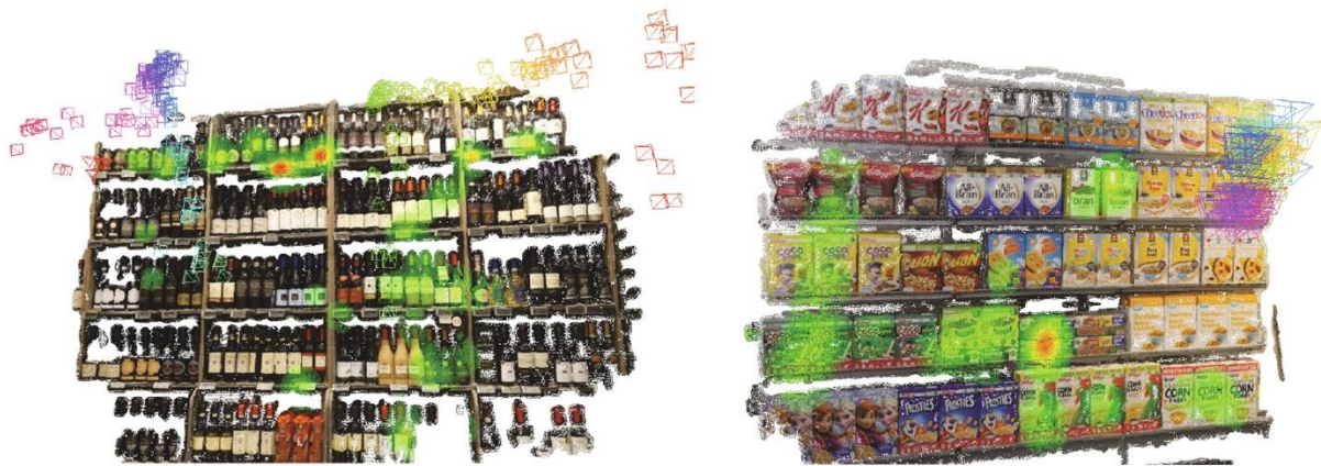
Fig. 3-3 3D gaze visualization result with the use of an extra RGB camera for 3D reconstruction [58]
