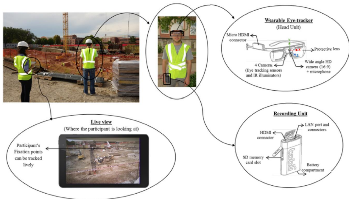
Fig. 1-5 Record the worker's visual attention by eye tracking glasses when the worker is working in the field [9].
