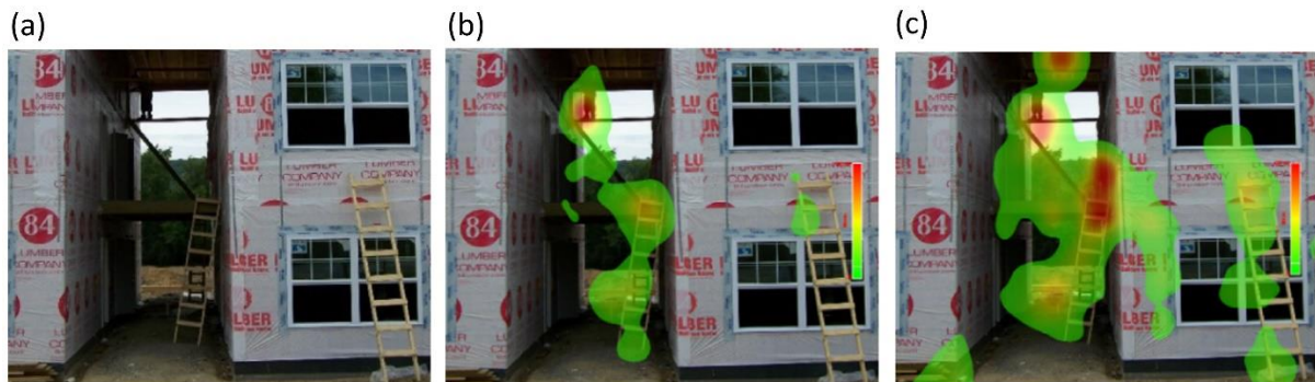
Fig. 1-4 Measuring impacts of safety knowledge on construction workers using eye tracking technology: (a) original picture, (b) attentional distribution for the group of less experienced workers (< 5 years), and (c) attentional distribution for the group of more experienced workers (> 10 years) [11].
