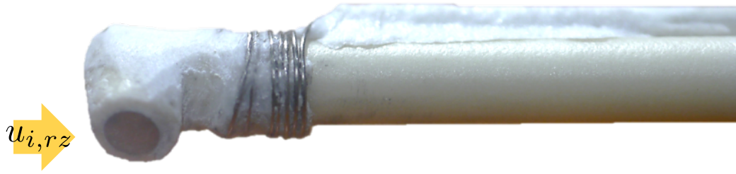
Figure 2.15: Photo of planar Langmuir probe.
