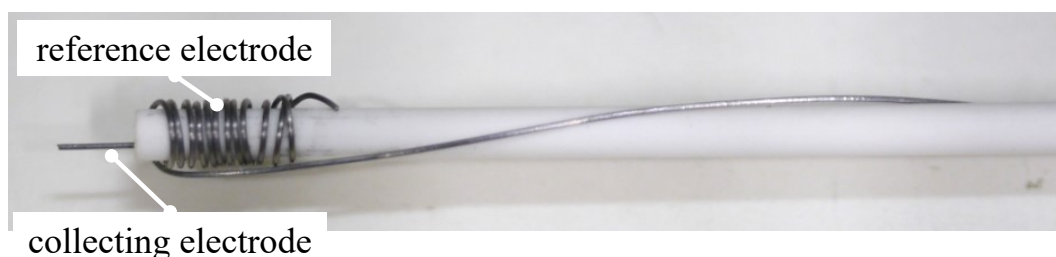
Figure 2.13: Photo of the RF-compensated Langmuir probe.
