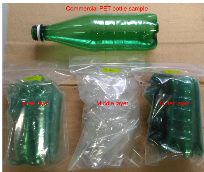
Figure 6-16: Separated layers of commercial PET bottle sample.
