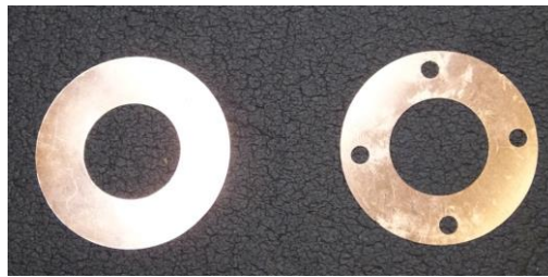
Fig. 3-13 A Inner fin for improvement of PCM heat conduction
