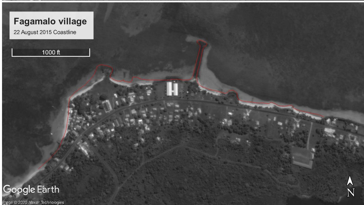
Figure 3.8 Satellite imagery of coastline change due to erosion in Fagamalo between 22 February 2003 (top) and 22 August 2015 (bottom). The red contour line indicates that the 2003 coastline that was eroded
