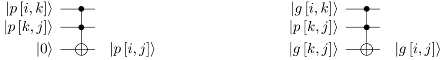
(a) A calculation circuit of p[i, j] as Eq. (6.5). (b) A calculation circuit of g[i, j] as Eq. (6.6).
