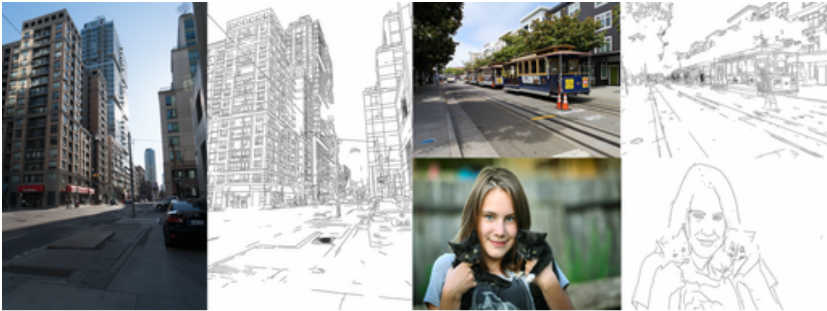
Figure 2.1: Examples produced by our model. Given an input photograph on the left, our model automatically generates a line drawing image on the right. The photograph of the woman is from svklimkin (Public Domain). (best viewed with zoom and in color.)
