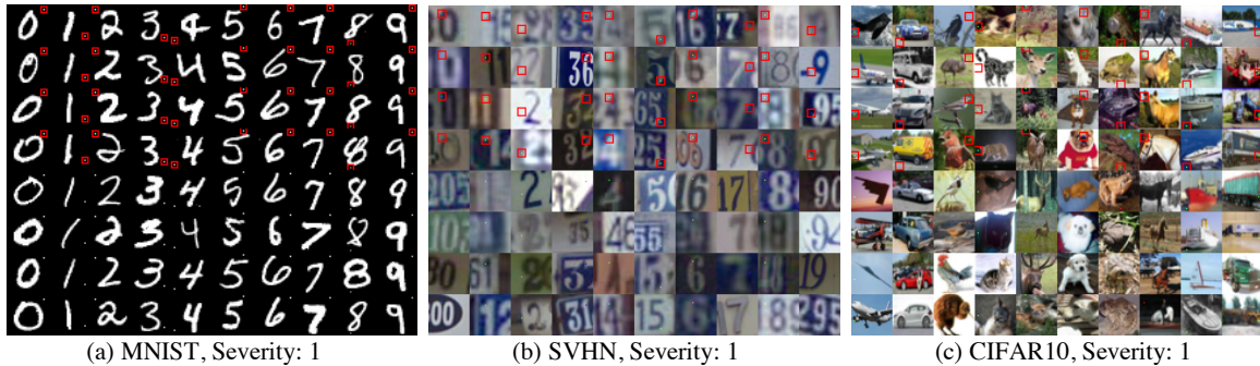
Figure 3-2: Perturbed training image samples obtained by the CMA-ES algorithm for single-pixel perturbation. The perturbed pixel locations are highlighted with red rectangles in the top five rows of the images.
