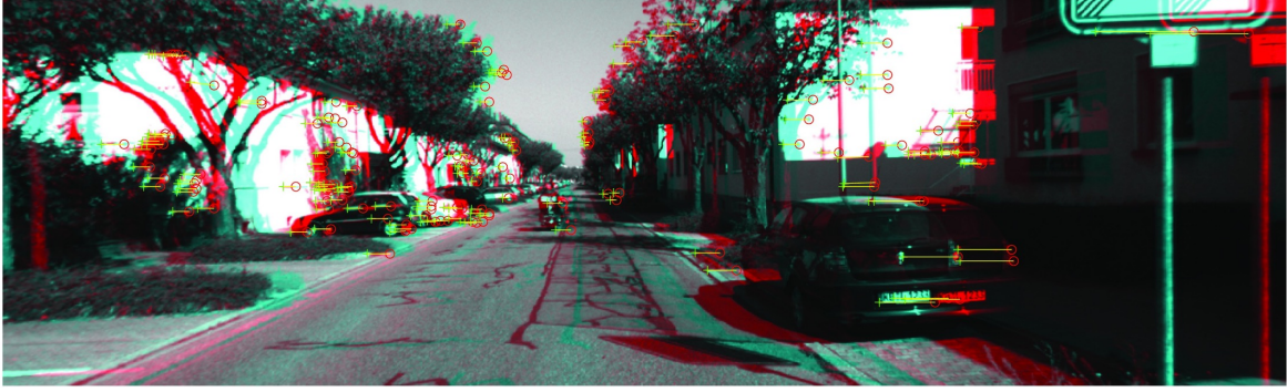
Figure 7.6 Stereo images overlaid from KITTI dataset. Since the stereo images are undistorted and rectified, the pixels matches are along parallel (horizontal) lines. Therefore, the disparity can be used to warp a image.
