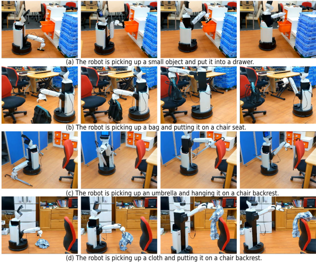
Figure 7.13: The HSR robot is tidying a room. (a) The robot is picking up a small object and put it into a drawer. (b) The robot is picking up a bag and putting it on a chair seat. (c) The robot is picking up an umbrella and hanging it on a chair backrest. (d) The robot is picking up a cloth and putting it on a chair backrest.
