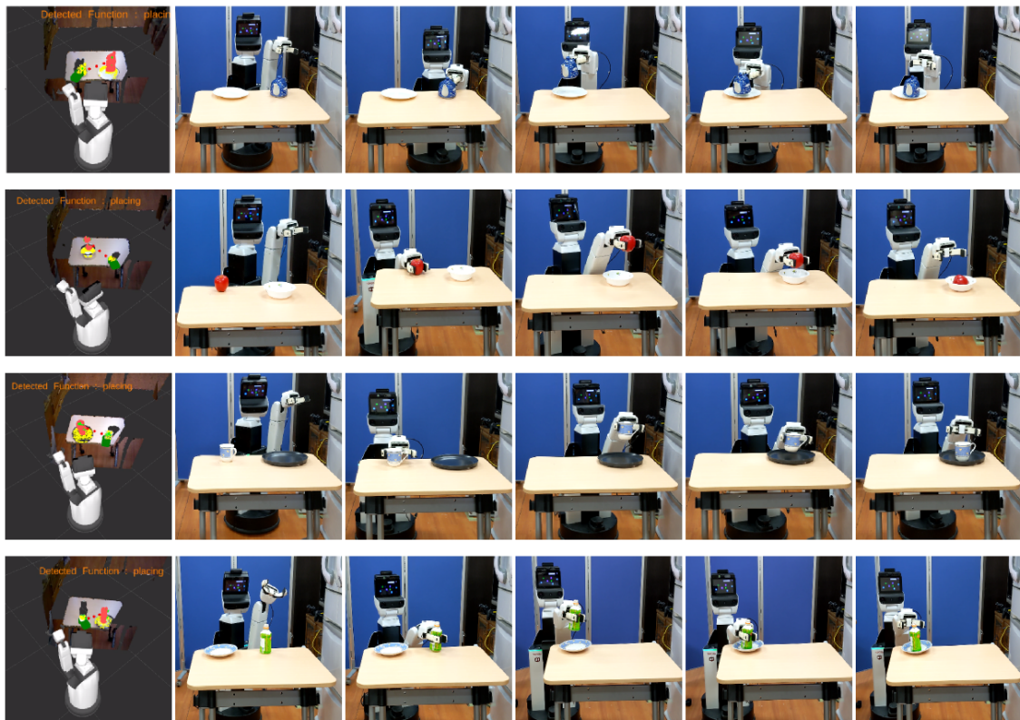
Figure 7.7: The HSR robot is performing the placing task using different object-pair combinations. First row: the robot picks up a teapot and puts it on the plate. Second row: the robot picks up an apple and puts it into a bowl. Third row: the robot picks up a cup and puts it on the plate. Fourth row: the robot picks up a bottle and puts it on the plate.
