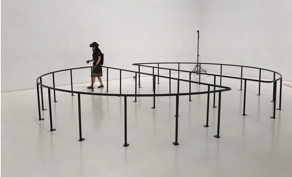
Fig. 7.8: Overview of Unlimited Corridor: Handrail Version. A user sees straight handrails through the head-mounted display (HMD) and feels that they are walking along gripping an ostensibly straight handrail, although they are actually walking along gripping a curved handrail.
