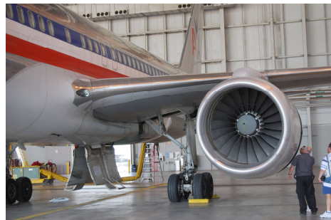
Fig. 1.1-2 An aeroengine mounted below an aircraft wing [2]
