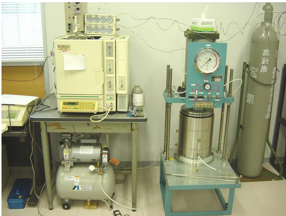
Figure 4.2-1 Equipments ( GC, compression machine, compressor, sample injector)
