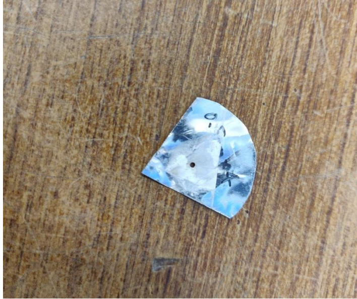
Figure 2.41 1 mm orifice plate
