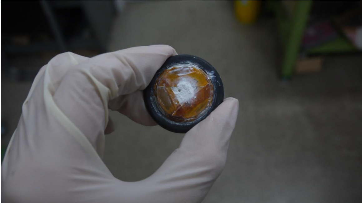
Figure 2.43 Orifice upstream side
