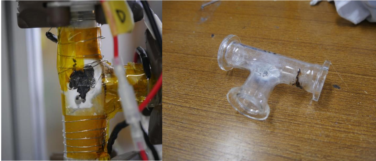
Figure 2.8 Damaged NW16 Nipple
