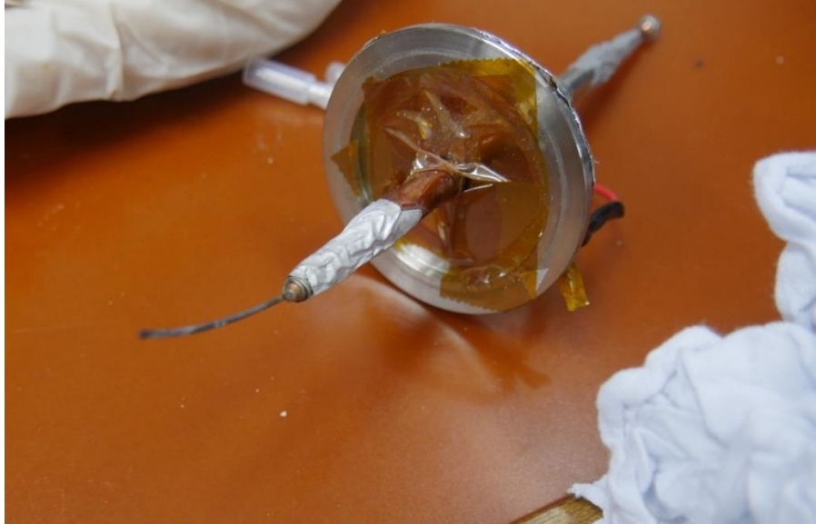
Figure 2.4 Discharge Electrode
