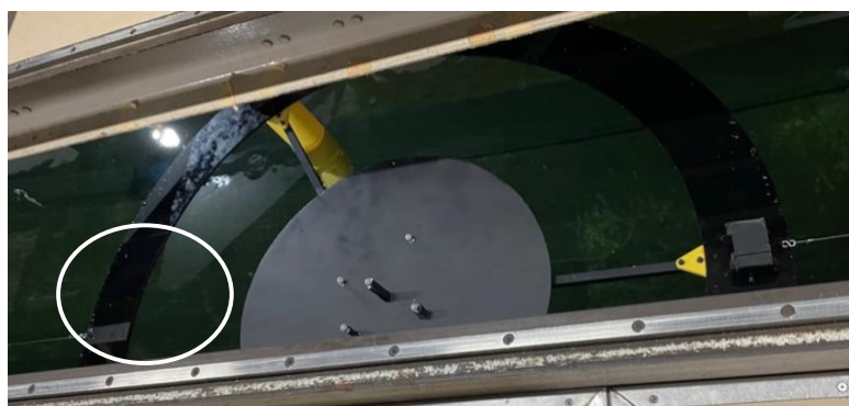
Figure 3-9 A case of the upper deck touching the water surface.
