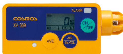
Fig. 2.4. The photo of the thermal-semiconductor-type detector utilized (COSMOS, XV-389)
