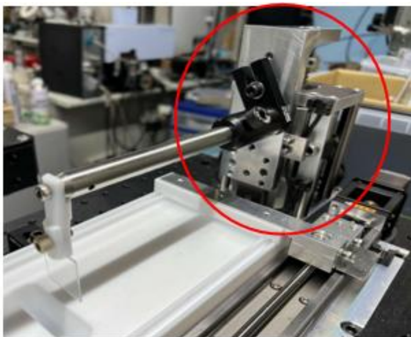
Fig. 3.3 Motorized lifter, used to lift or immerse solid substrate.
