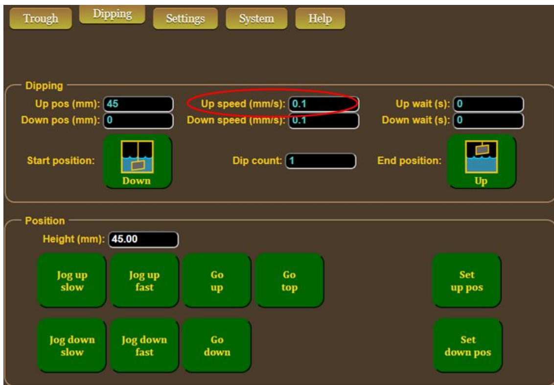
Fig. 3.7 The dipping page of the LB controller. Inside the red circle is the crucial lifting speed parameter (Up speed).
