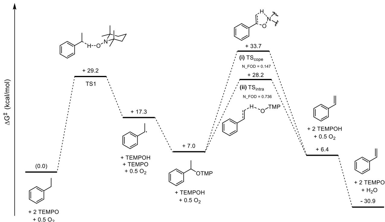
**Figure 2.** Computed free energy profiles for the aerobic dehydrogenation of **1a** to **2a**. The DFT Calculation was performed at FT-TPSS-D4 (5000K)/def2-TZVP//FT-PBE0-D4 (10000K)/def2-QZVPP level of theory.
