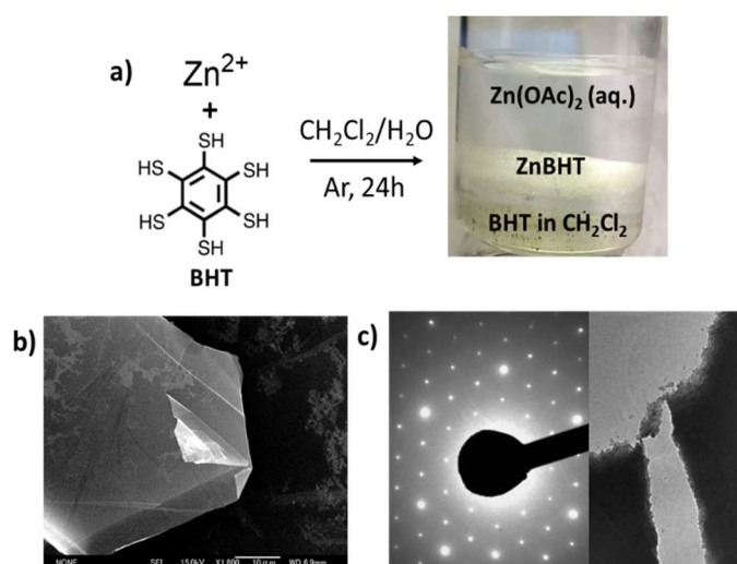
Figure 1. a) Liquid-liquid interfacial synthesis of ZnDT ; b) SEM picture showing layered ZnDT ; c) TEM and SAED pattern implying hexagonal lattice in ZnDT .
