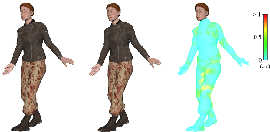
Figure 3.12: Comparison of ground truth (left), prediction results via DenseGATs (center), and color map (right) indicating per-vertex distance error.
