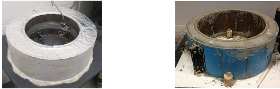
Figure 1.4 (a) the covered dual ring and (b) the uncovered dual ring
