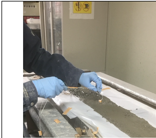
S3. Placing Temperature sensors
