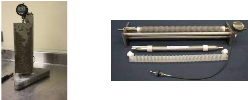
Figure 1.3 (a) Experimental set-up for ASTM C157 standard (b) ASTM C1698 standard
