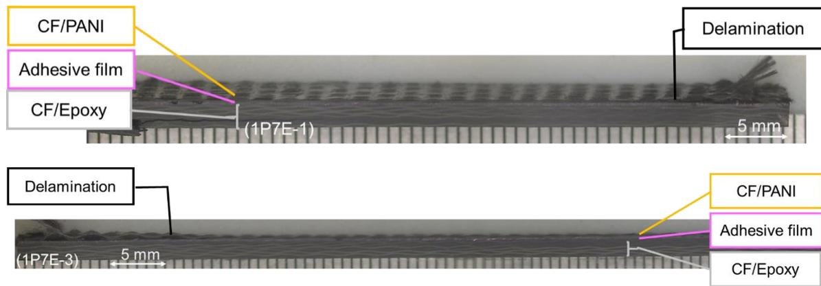
Figure 4-23 Delamination at the edges of CF/Hybrid-1P7E of specimen number 1 and 3 (Centre parts)
