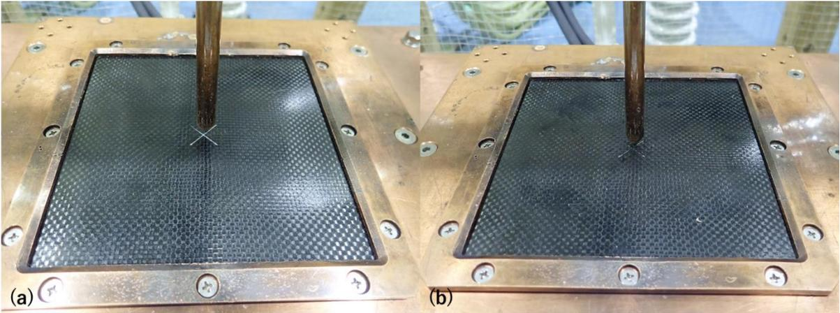
Figure 4-4 CF/Hybrid-4P4E before and after lightning strike (a) before and (b) after lightning strike
