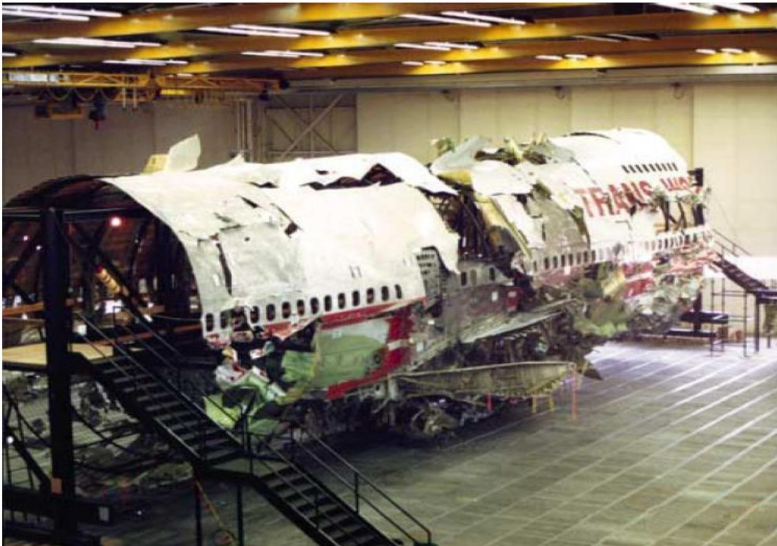
Figure 1-4 Reconstructed wreckage of TWA 800 [5]
