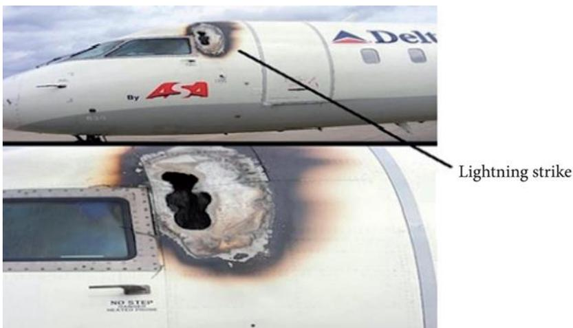
Figure 1-3 Lightning strike damage on aircraft [3]
