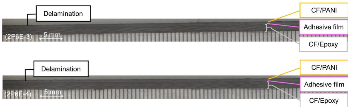
Figure 4-16 Cross-sectional images of CF/Hybrid-2P6E after lightning strike at 15 mm and 30 mm from the centre
