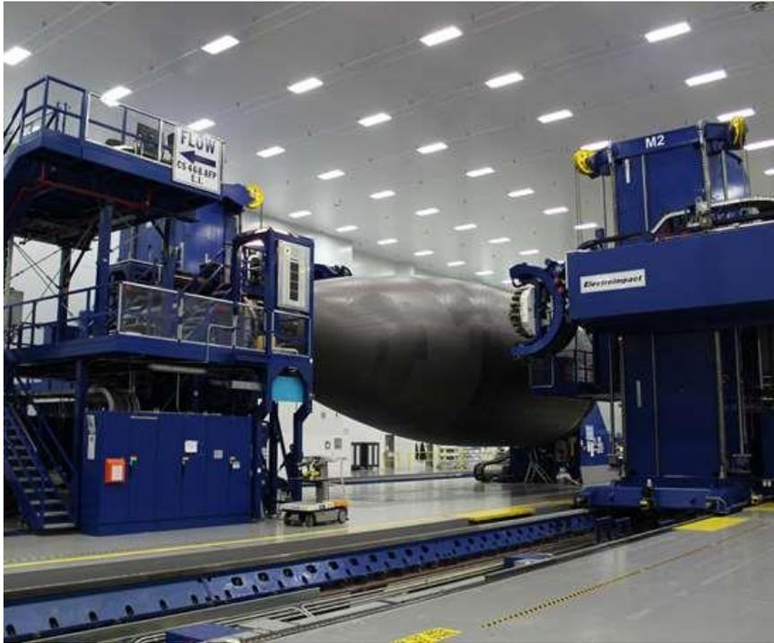
Figure 1-2 Forward Fuselage of Boeing 787 made of carbon fibre composite structure [2]
