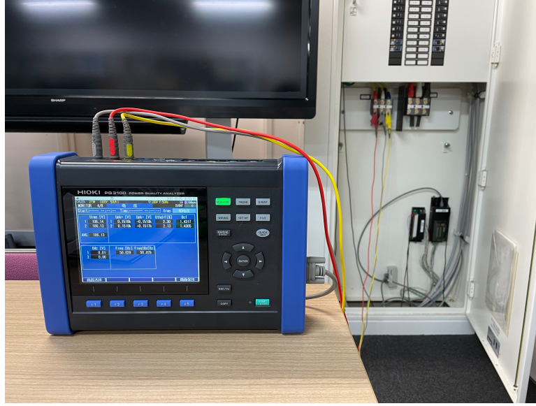
FIGURE 4.13: Measuring system frequency with a power quality analyzer.
