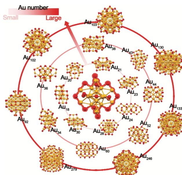
**Figure 5.** Stable gold nanoclusters with different core size indicated, reported until 2018. Central cluster, Au<sub>25</sub>SR<sub>18</sub>, consists of 25 gold atoms.<sup>14</sup>
