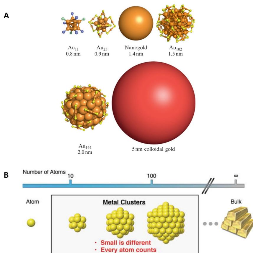
**Figure 1.** A: Gold nanoclusters and gold nanoparticles compared <sup>2</sup>. B: Relation of gold clusters, gold atoms and bulk gold <sup>3</sup>.
