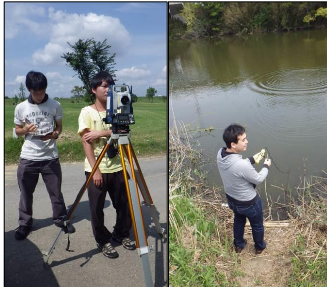
Figure 3.24. Field Measurement Using Total Station and Depth Measurement Device
