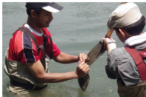
Figure 3.30. Sample collection on riverbed by using Ekman Berge (left) and Scoop (right)
