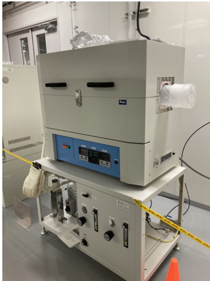
Figure4.6 The thermal oxidation furnace.
