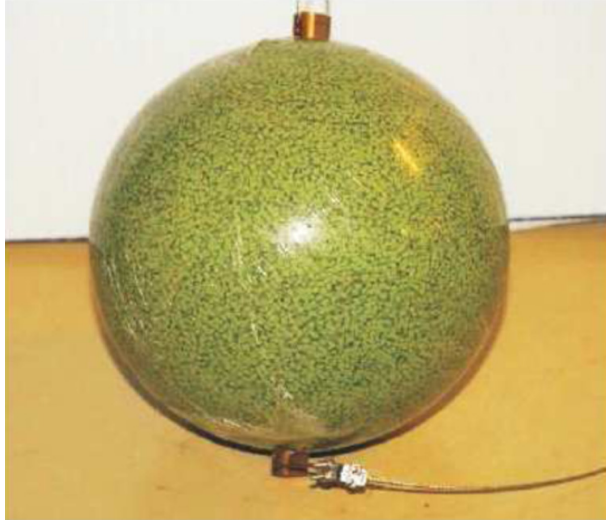
Figure 4.2: Picture of Ni-Cf source. This ball is made of 6.5 kg of NiO and 3.5 kg of polyethylene. The Cf source (neutron source) was inserted into the center of the ball. Taken from [80].
