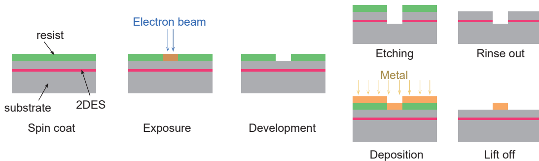
Figure 3.2: Procedure of Electron-beam lithography. After development, the process can be divided into two types; namely etching and deposition.
