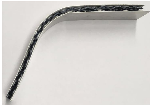
Figure 2-27. Deformed sandwich sheets with A2017P faces at clearance of 15 mm.
