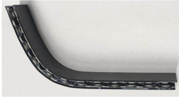
Figure 2-31. Deformed sandwich sheets with CFRTTP faces at clearance of 15 mm.
