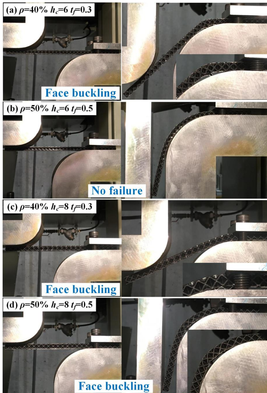
Bending of sandwich sheets with the octet plate core
