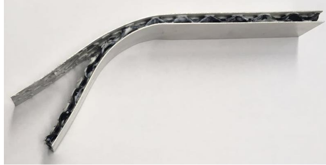
Figure 2-25. Deformed sandwich sheets with A2017P faces at clearance of 8 mm.
