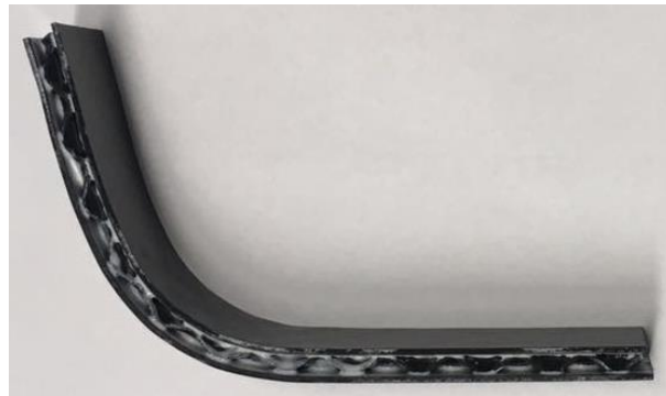
Figure 2-29. Deformed sandwich sheets with CFRTP faces at clearance of 8 mm.
