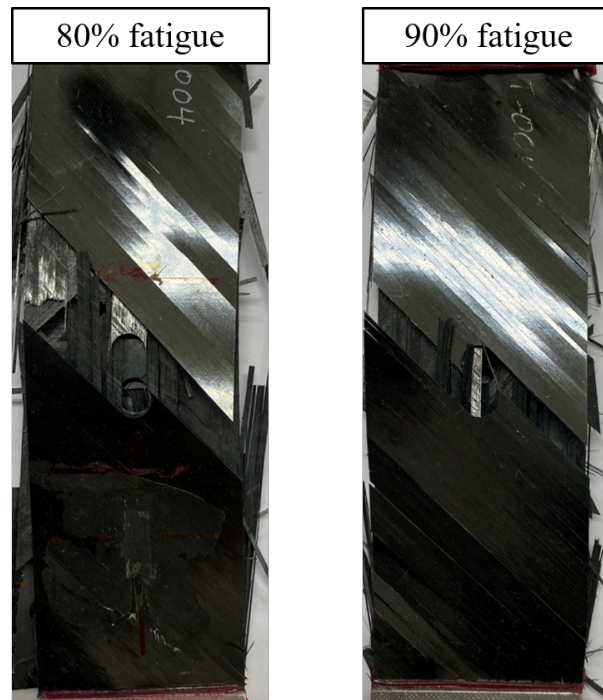
Fig. 5.3 Failure specimens of [+45_4/0_4/-45_4/90_4]_{2S} laminates : 80% and 90% fatigue conditions.
