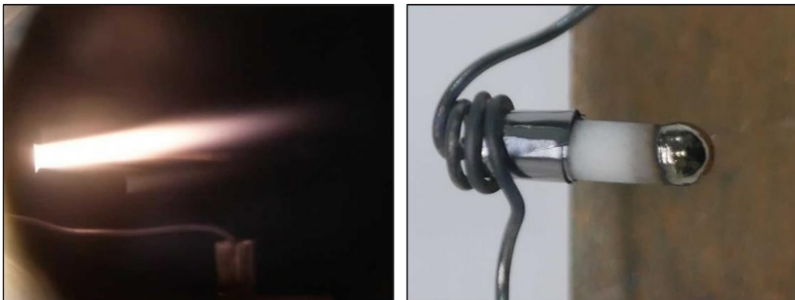
Figure B-2 Photographs of ablation plume (left) and zirconia rod after laser ablation (right).
