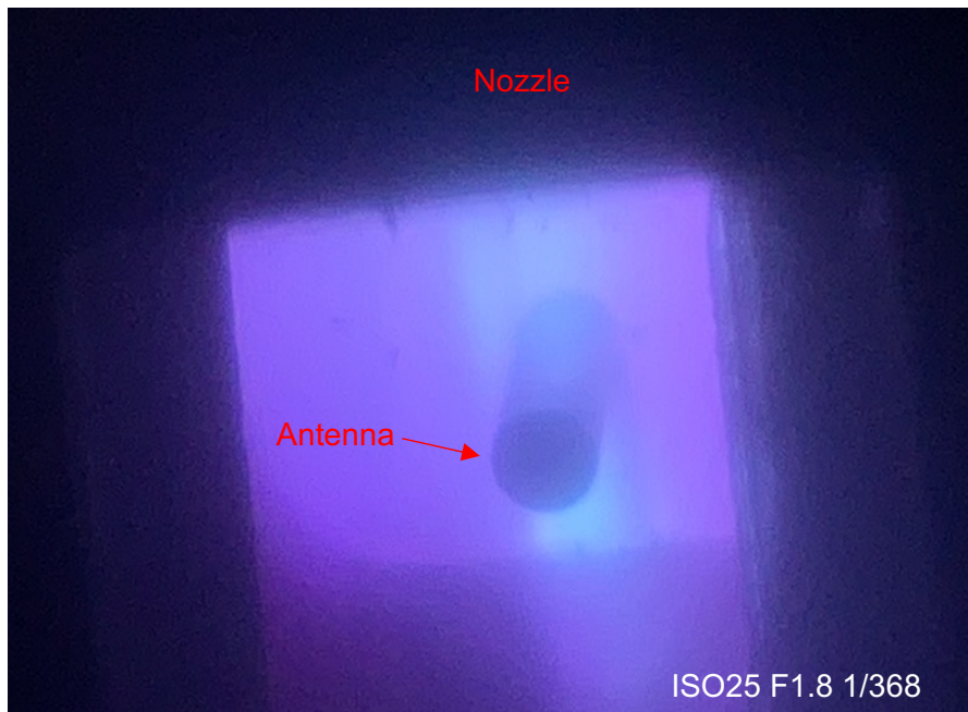
Figure 3.29: Optical observation of internal plasma with the antenna facing the optical window for the nominal conditions.
