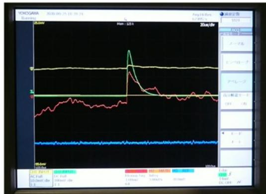
**Fig. 2.21** Transition of TALIF signal with respect to the number of average. Green line: laser signal detected by PMT2, red line: fluorescence signal detected by PMT1 in Fig. 2.19
