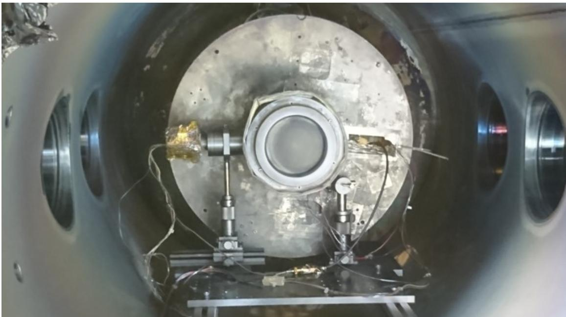
**Fig. 2.11** Front view of thruster. Laser was injected from the bottom window.
