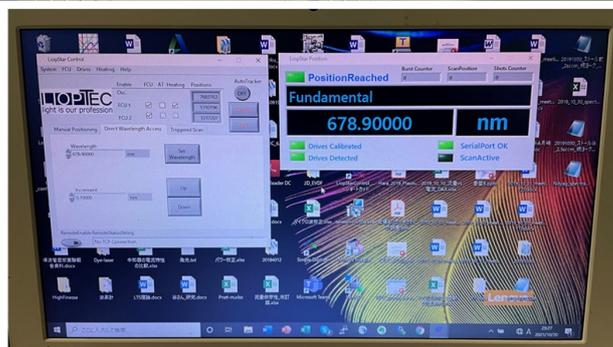
**Fig. 2.14** Dye laser system. This dye laser converted to the wavelength from 532 nm to 650 ~ 700 nm by using dye, and the three harmonic light was extracted. A laptop can operate dye laser system, for example, the changing wavelength.
