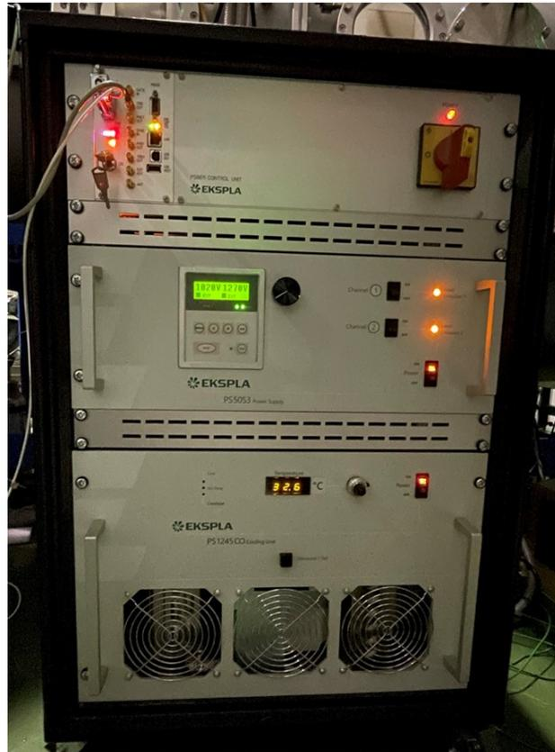
**Fig. 2.12** Power supply of Nd:YAG laser. In this thesis, two times harmonic wavelength of 1064 nm, i.e., 532 nm, was used.
