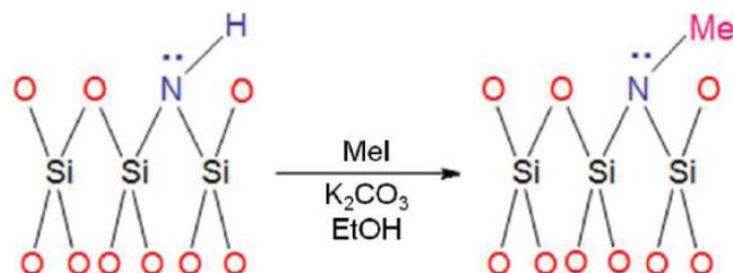
Figure 1-12 Methylation of nitrided mesoporous silica.[71]
