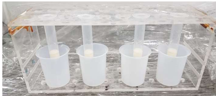
Figure II-3. Purification system of seawater using Nobias chelating resin syringe.
