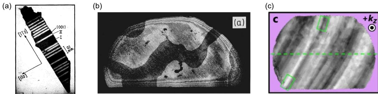
Figure 4.3: (a) Orientational antiferromagnetic domain pattern in NiO visualized by LB-based imaging. (b) SHG image of a antiphase domain pattern in Cr<sub>2</sub>O<sub>3</sub>. Sample size is  $6 \times 3$  mm<sup>2</sup>. (c) NLD image of an antiphase domain pattern in Pb(TiO)Cu<sub>4</sub>(PO<sub>4</sub>)<sub>4</sub>. (a), (b), and (c) are taken from Refs. [74], [75], and [76], respectively.
