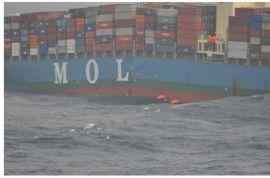
Fig.1.2 MOL COMFORT の破断事故 [2]
