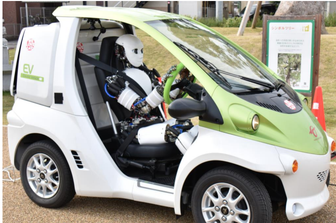
Fig. 7.63: Autonomous driving by the musculoskeletal humanoid, Musashi [271].
