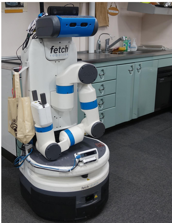
Fig. 4.3: Fetch: The mobile robot with an axis-driven single arm.
