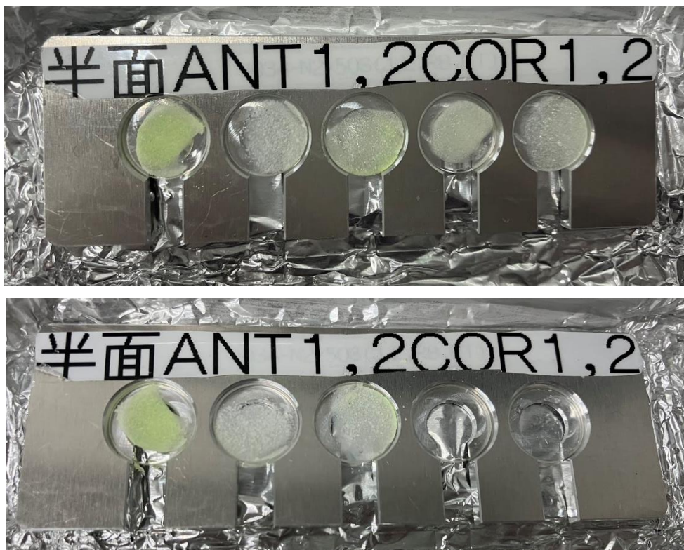
Figure 3.2.3 Anthracene samples before (Top) and after (Bottom) irradiation of deuterium arc lamp.
